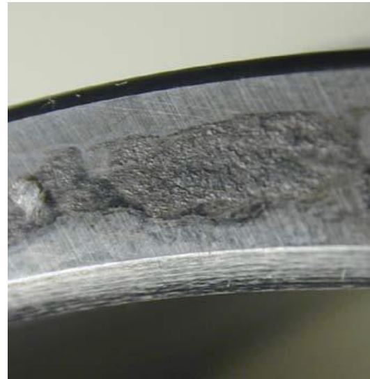
Outer ring: Fretting corrosion on the side face
