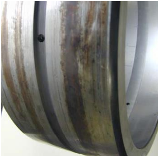
Outer ring: Fretting corrosion on the outside surface
