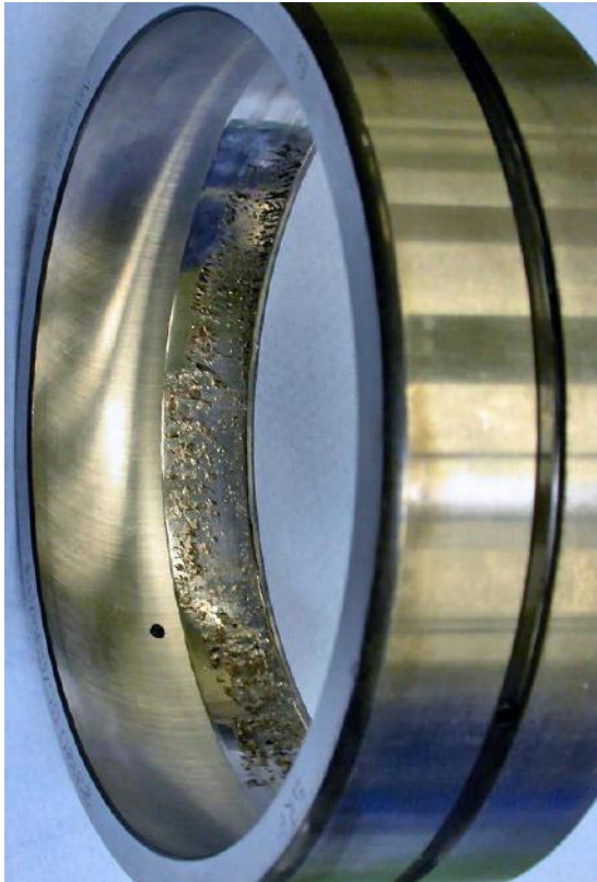
Spalling in the outer ring raceway
