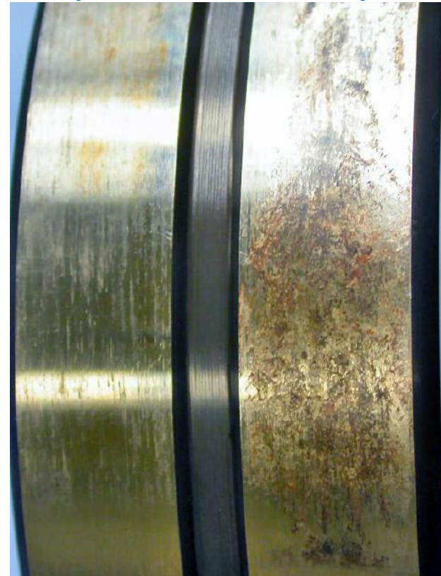
Damage to the outer diameter surface
