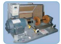
Considerable time shall be dedicated to hands-on practical sessions, taking vibration data and simulating machinery faults including unbalance, misaligment, losseness, bent shaft, rubbing and bearing damage.
